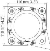
Adjust screws to change horizontal and vertical tilt angle (max 5°)
