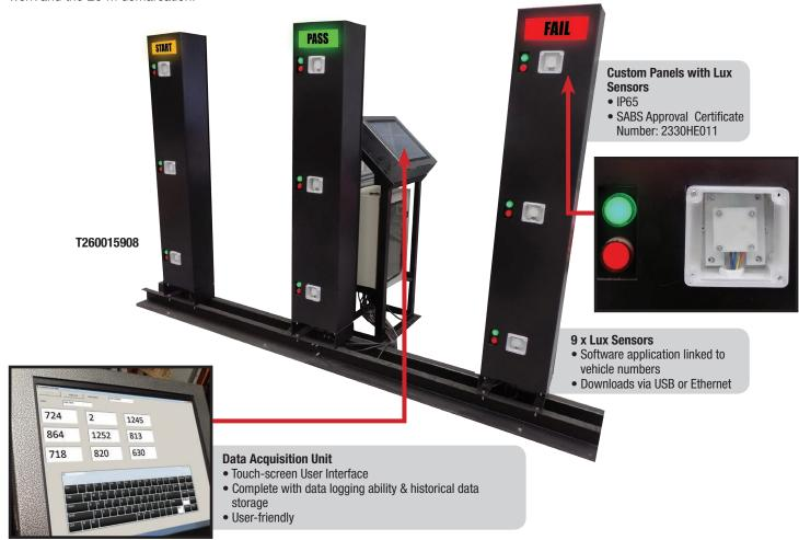
The system will be activated by the vehicle operator at the 20 m area, either by manual or automatic input, once our system receives this command ID the actual lux testing will commence, this will be confirmed by an amber light – START, once the test has been completed the system will give either a green light – PASS, or a red light – FAIL indication.
