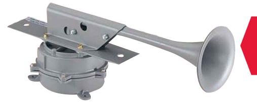
The **Federal Signal Model 52** resonating horn produces 114 dB @ 10 feet (124 dB @ 1m) with a 1,000 foot (304.8 m) range. It is capable of penetrating high ambient noise levels. Being electrically activated, the Model 52 does not require an air compressor for operation. The **Model 52** is able to withstand the shocks, vibrations, dust and atmospheric conditions encountered in off-road use. The operating temperature range is -40°F to 185°F (-40°C to 85°C).
