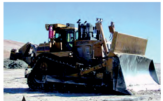
D10R with very high CFM requirements has a quadruple OPTIMAX installation
