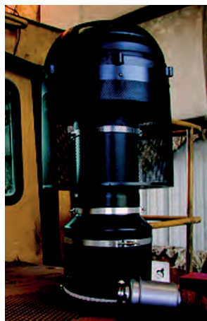
D10R with very high CFM requirements has a quadruple OPTIMAX installation
