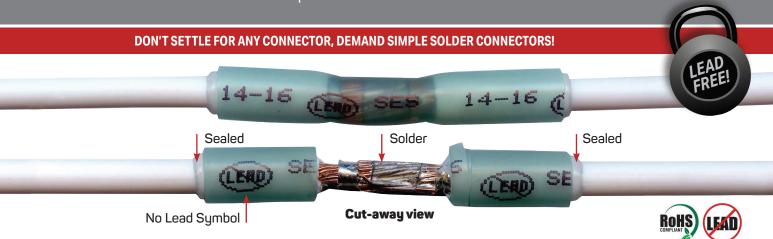
Simple Solders' Connectors are a revolutionary new wiring connection system for cable connections and end terminations. The best electronic and electric equipment available on the market becomes useless if not connected properly. Simple Solders provide a high-quality, sealed solder connection that takes the guesswork out of soldering. Soldered terminations provide superior tensile strength and conductivity.
